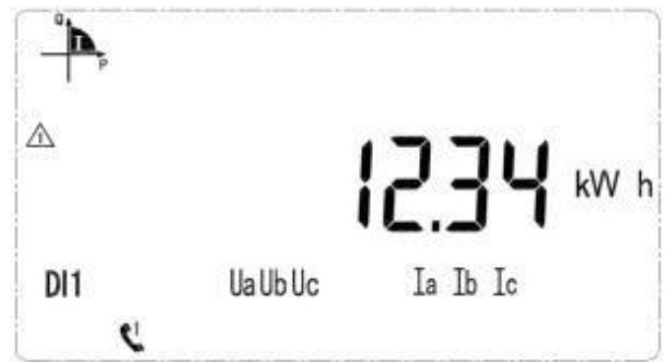
Current reversing active energy 12.34kWh
