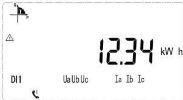
Current forward active energy 12.34kWh
