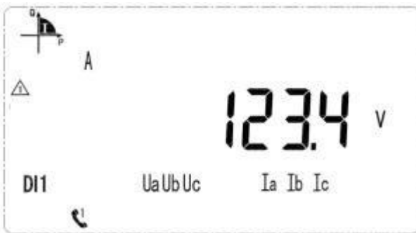
Voltage on A phase is 123.4V
