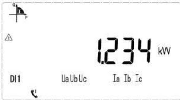
Current total power is 1.234kW
