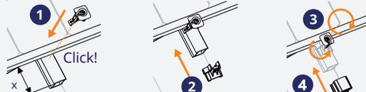
1. Place the module clamp onto the rail.
