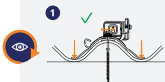
1. The feet of the mounting brackets should rest in the troughs.
