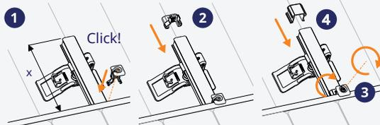
1. Secure the module clamp to the rail.
