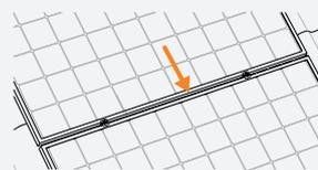
**⚠ Note:** Make sure the solar panels are aligned before you tighten the screw.
