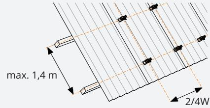
Only use the (existing) roof screws in the positions indicated by the corrugated sheet supplier. Screws should not be used in different positions. Exclusive mounting on corrugated sheet's rise and right above the purlin.
