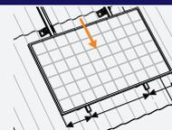
**⚠ Note:** Click the cables into the cable clip and slide the panel to the bottom of the rail.
